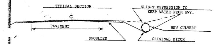
Six inch minimum gravel cover over culvert
