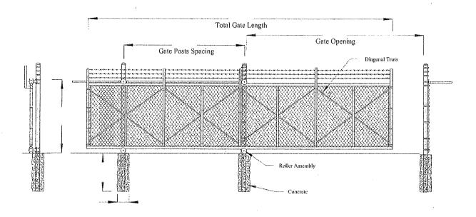
Note: Diagonal Braces can be Truss wires, Truss Rods or Tension Bars.
