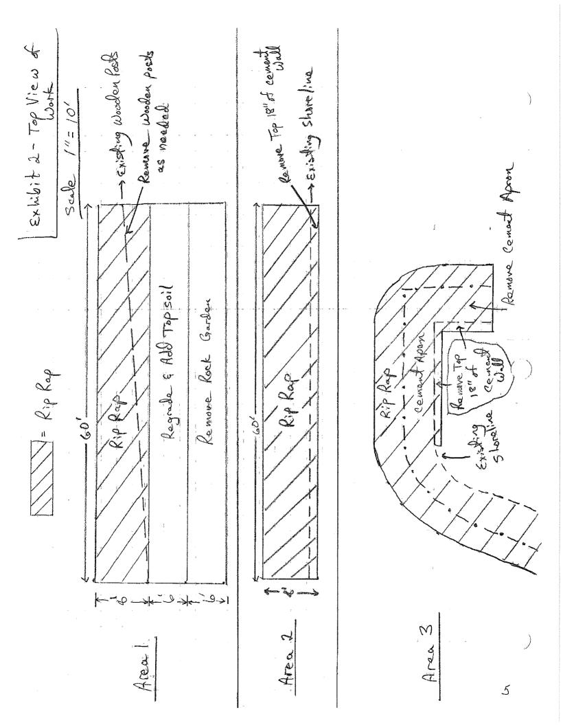
Exhibit 3 - Cross Section Regrale & Scale Add Top Soil Area 1 1= Rip Rap Remove Wooden Posts as needed Rip Rap Fill & Rocks Area 2 Remove top 18" of cement wall Rip Raps Area 3 Remove top 18" of cement wall Rip Rap
