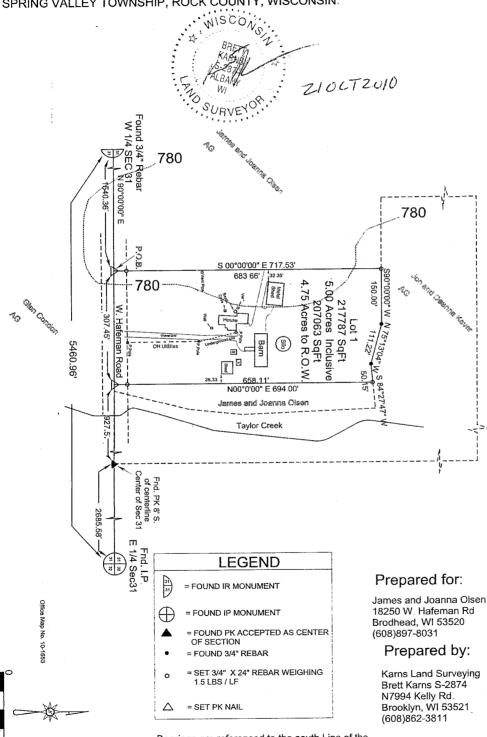
Bearings are referenced to the south Line of the E-W 1/2 line of Sec 31, T2N, R10E, town of Spring Valley, Rock County, WI, assumed to bear N 90°00'00"E.
