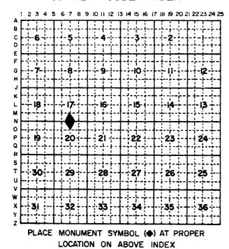
1. Above code numbers are positioned Meander, Claim, or Fractional corners of the section.
