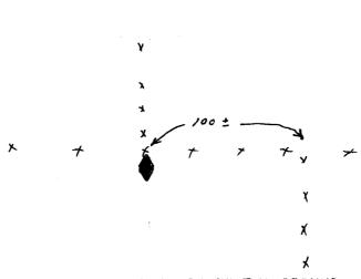
FOUND CUT LIMESTONE 0.1' BELOW THE GROUND. STONE IS 0.7' S OF CORNER FENCE POST. SET CARSONITE ON E SIDE OF STONE.
