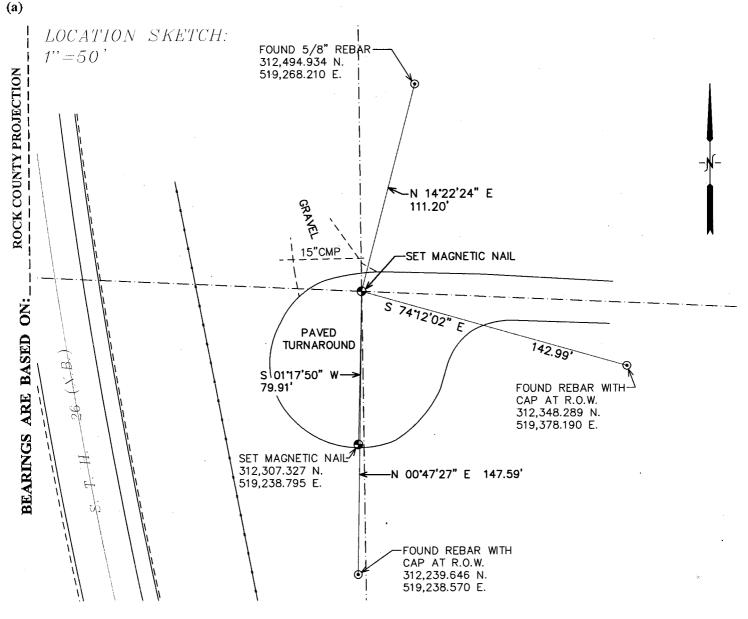
FIELD BOOK \_\_\_\_\_ PAGE # \_\_\_\_ OF OR OBSERVATION SHEET \_\_\_\_ OF \_\_\_ SHOW A PLAN VIEW DRAWING DEPICTING THE CORNER MONUMENT AND SURROUNDING PHYSICAL FEATURES, INCLUDING THE EXCAVATION AREA AND DEPTH.
