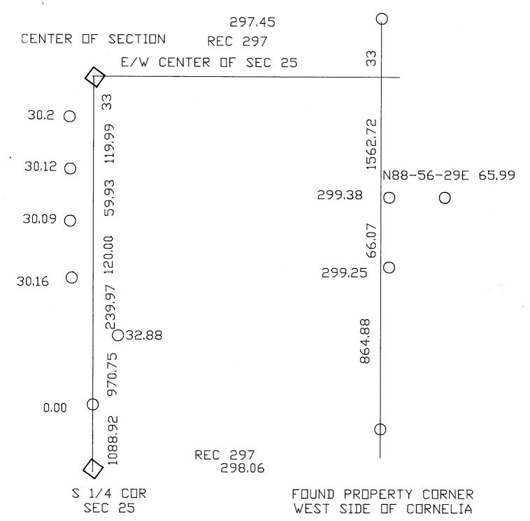
DISTANCES NEXT TO PROPERTY CORNERS REFLECT THE OFFSET DISTANCE FROM THE CENTER OF SECTION TO THE SOUTH QUARTER CORNER OF SECTION 25.
