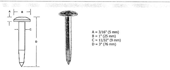
The Steel Nail Marker is super strong solid steel and drives easily into blacktop. "SURVEY MARK" is imprinted on top of nail for easy identification as a survey mark. The SNM1 has a 1" (25mm) convex top and conical recessed center chamfer for pinpoint accuracy.
