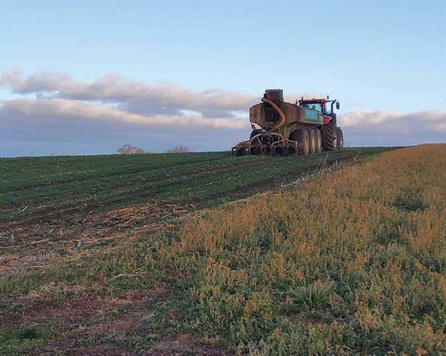
Photo: Application of manure using low-disturbance manure injection on a fall-planted winter rye cover crop following corn silage.
