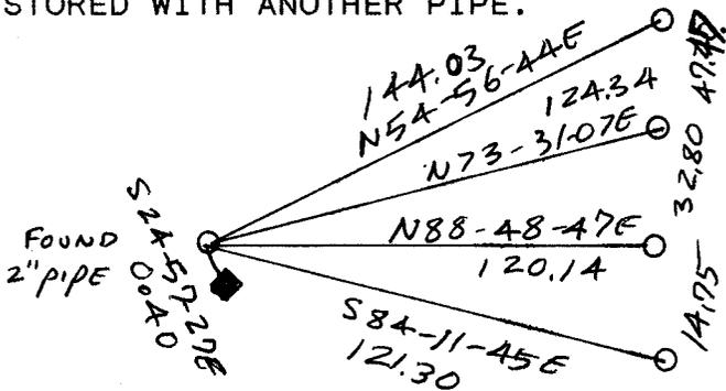
(e.) Was the corner reestablished through lost corner proportionate methods? If so, show the method, including the directions and distances to other public land survey corners used as evidence or used for proportioning in determining the corner location.
