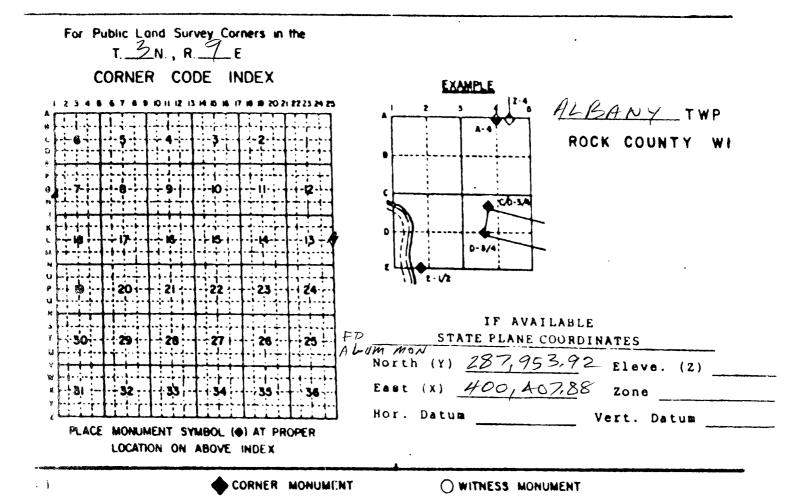
COORDINATES ARE ENSED ON THE ROCK COUNTY PROJECTION SYSTEM. ESTABLISHED BY CONVENTIONAL TRAVERSE FROM GPS "ALBANY" 304S AND THE AZIMUTH "ALBANY AZIMUTH" 304A WHICH IS IN THE SW 1/4 OF SECTION 7.
