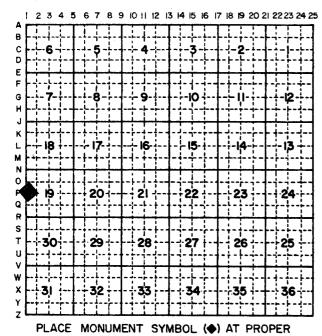
Above code numbers are positioned Meander, Claim, or Fractional corners of the section.
