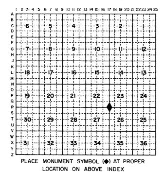
1. Above code numbers are positioned Meander, Claim, or Fractional corners of the section.
