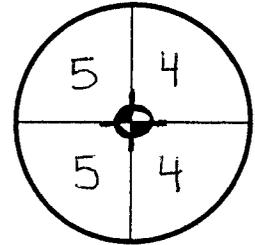
Location Sketch, showing corner identification name with references to at least four accessories, fence or occupational lines, centerlines of roads, and other site details for reference. If in disagreement with previously established corner, distances are shown between the two corners with references to the disputed corner from the accessories.
