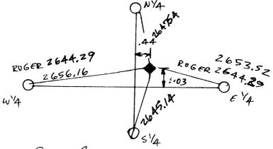
le Barres , hereby certify that the corner points as identified by the corner code index were, in a field survey on S695 1985, established, re-established, monumented, re-monumented, recovered or restored as expressed below and in conformance with the regulations and rules as required in the current manual of survey instructions of the United States Department of Interior, Bureau of Land Management.
